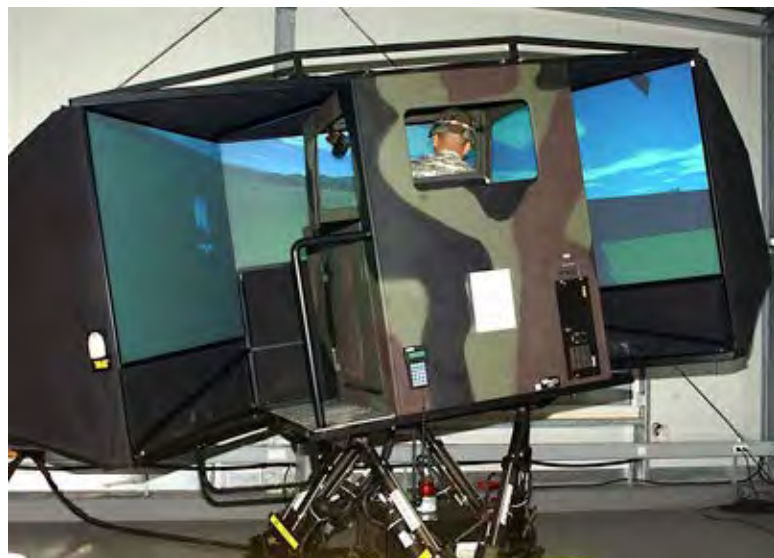
Heavy vehicle simulation at Dexheim, Germany
