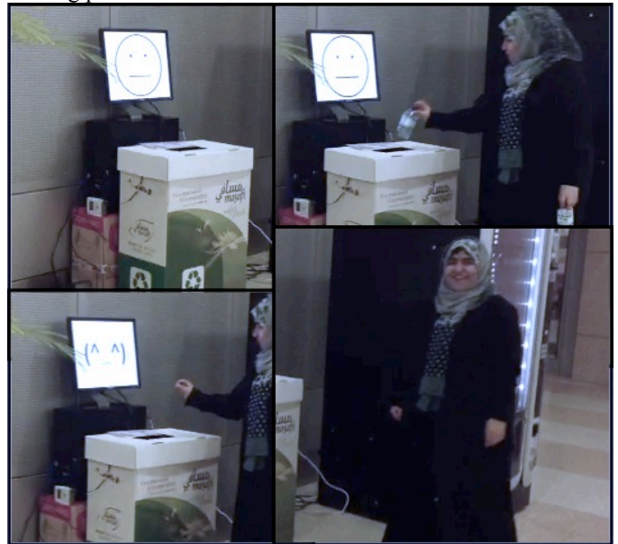
Figure 1. Student recycling with emo-bin. The LCD poker face changes to happy each time a user feeds a bottle. Compared to a standard bin, recycle rates go up x3 times.
