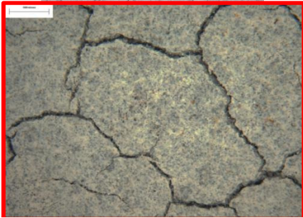
High Build Silicone 1 First sign of cracking 300°C
