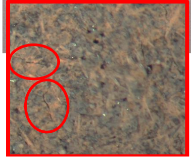
Experimental High Build Silicone First sign of cracking 650°C
