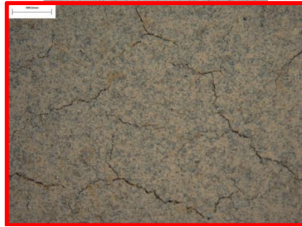
High Build Silicone 2 First sign of cracking 400°C
