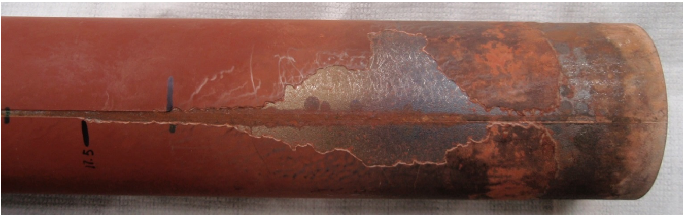
Figure 14: A pipe with 3x100 \mu\text{m} Epoxy Mastic after exposure in the modified Houston piep test. The delamination from the scribe was determined with the tip of a knife to extend to approx. 17.5 cm from the end of the pipe corresponding to a temperature of 153 ^{\circ}\text{C} .
