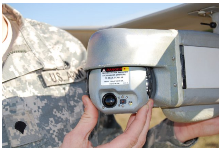
The new RQ-11B Raven gimbaled payload upgrade allows for greater ease of flying providing 180-degree panning of the infrared/electro-optical camera and laser illuminator
